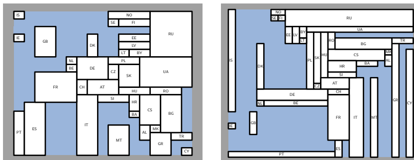
Fig. 2. Two rectangular duals of the dual graph of a map of Europe (from [2]).
