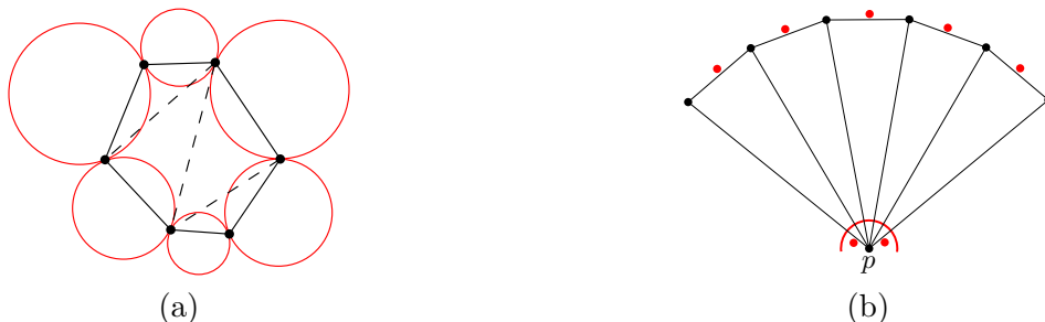
Figure 2: (a) At least n points are required to block this n -vertex Delaunay triangulation. (b) This n -vertex Delaunay triangulation can be blocked by n points.
